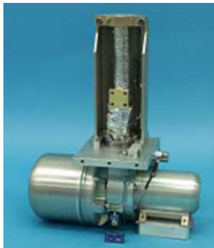
Figure 4.3—Two stage conventional 20 K flight cryocooler used in GRC ground testing.
