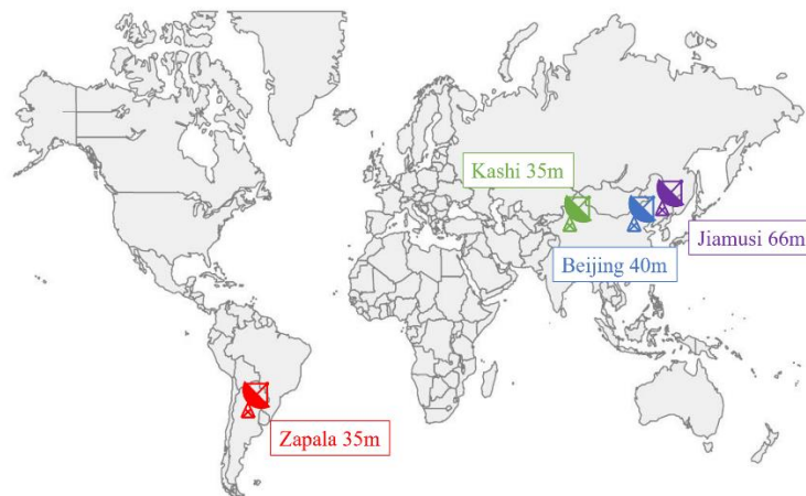
Figure 4. The deep-space network of China can basically achieve full coverage of the data
