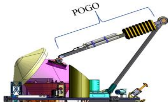
Figure 2 - Single Plane of Motion TAGSAM with potentiometers for simple & reliable positioning
