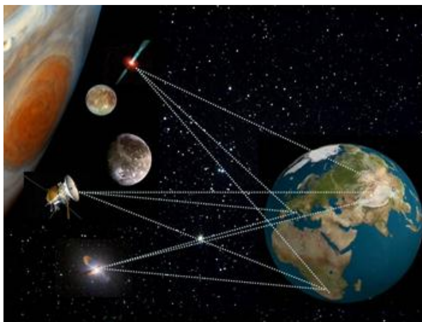
Figure 4-26. Generic PRIDE configuration. The Earth-based segment of PRIDE combines a network of VLBI radio telescopes and data processing centres.
