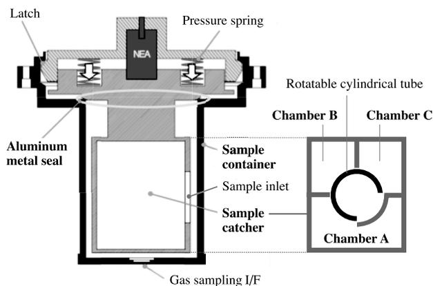
Fig. 6. Schematic illustration of the Hayabusa2 sample catcher and container.
