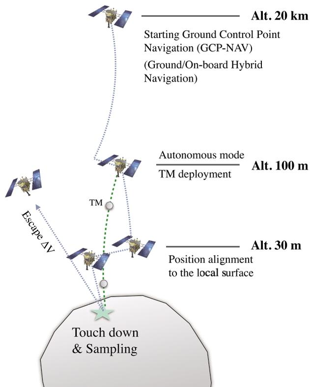
Fig. 7. Operation sequence for touchdown and sampling.
