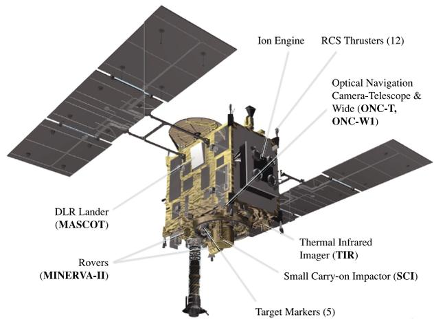
Fig. 2. Illustrations of the Hayabusa2 spacecraft with instrument names.
