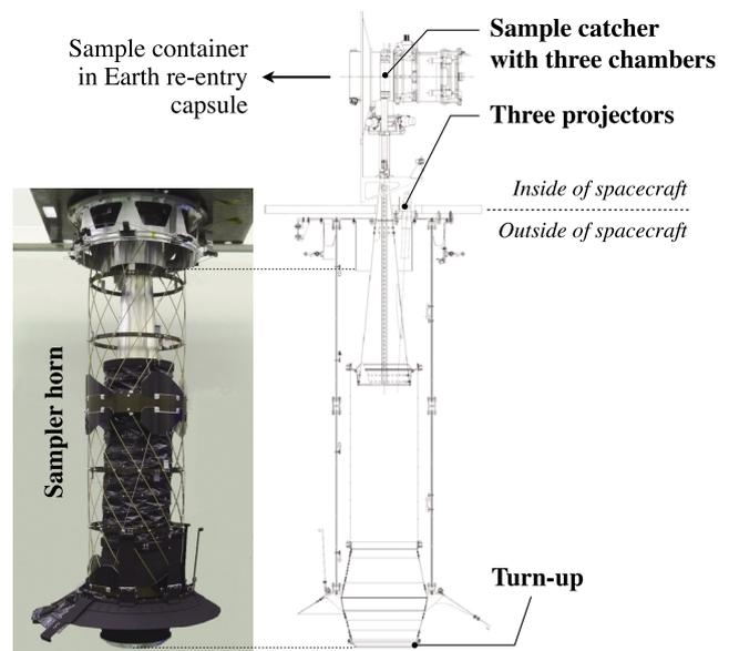
Fig. 5. Photograph of the Hayabusa2 sampler horn and schematic illustration of the Hayabusa2 sampler.
