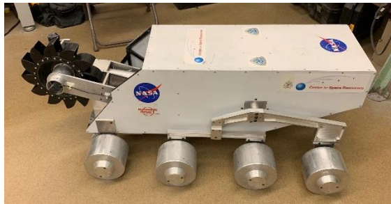
Mike Duke/ Colorado School of Mines Bucket Wheel Excavator
